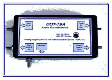
The **DOT-19A** was designed to protect traffic cabinets from catastrophic electrical surges and high frequency noise. The **DOT-19A** employs Series Hybrid Inductor circuitry, which also provides an excellent degree of filtering. In addition, a status indicator light allows the user to monitor the integrity of the suppression elements. This feature helps eliminate damage to traffic controllers due to degraded or failed surge suppression components.
