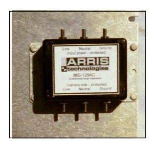
The IMG-120AC is a multi-stage hybrid surge protector intended for traffic camera AC power (120V) applications. The primary feature of the IMG-120AC is its symmetrical hybrid circuit topology, which consist of MOV banks on each side of series inductors. This design provides equal protection for surges emanating at the AC power mains (protects camera and adds additional surge suppression capacity to cabinets main filtering) and for surges produced at the remote camera (protects cabinet).
