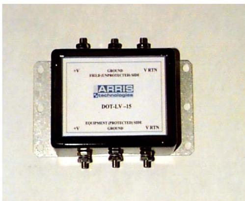
The **DOT-LV** power protection system employs a multi-stage hybrid suppression circuit designed for low voltage, high exposure applications. Metal oxide varistor and silicon avalanche technology is utilized to provide high surge capacity and low clamping voltage in an industry standard package.
