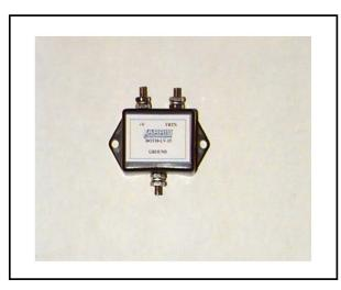
The **DOT10-LV** power protection module is a single-stage suppression circuit designed for low voltage, low/medium exposure applications. High power silicon avalanche technology is utilized to provide high surge capacity in a small footprint package. The small package allows close proximity placement to the device being protected, preserving the DOT10-LV's response time and clamping level by reducing inductive lead length effects.
